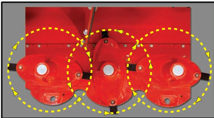
The blade overlap has been specifically designed by Capello engineers for a clean and even cut, even in the most dense and wet products. The blades are changed with a quick-change tool – no other wrenches needed. Each disc is protected by an individual shear spline in each disc to protect the remainder of the cutter bar in the event of a damaging impact with a field obstruction.
