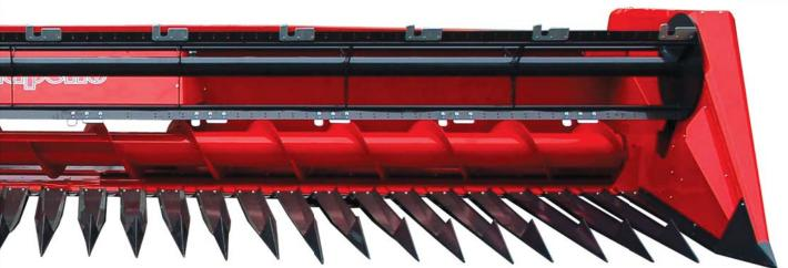
The auger is designed as a single-piece component and requires no additional support hardware for the entire length. This provides for more even product flow to the feeder channel, even in difficult field conditions. The auger drive is protected by a slip clutch that prevents gearbox damage commonly caused by foreign objects or collisions.
